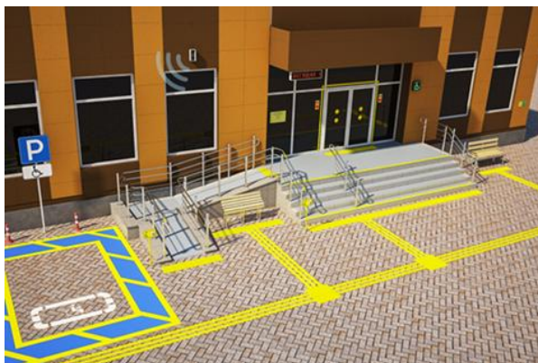
Figure 4. An equipped entrance for the disabled.
